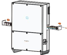
**Step 9** Press the hump of the latch hook and unplug the cable connection joint outwards.
