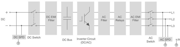
Fig. 2-4 Main Circuit Diagram
