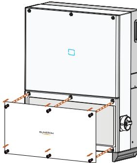
**Step 5** Measure AC voltage to ground at the AC terminal to confirm AC output of PCS at the AC circuit breaker is voltage free.
