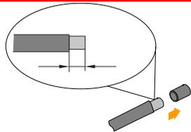
**Step 3** Insert the end of the DC cable to the cable socket that matches with the M10 bolt and tighten it with the proper tool.
