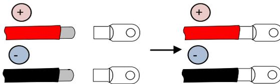
**Step 4** Install the heat-shrinkable tubing, shrink the tubing with hot air blower.
