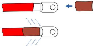
**Step 5** Loosen the swivel nut of the gland terminal (Marked as “BAT. Input”) and select an appropriate seal according to cable outer diameter. Lead the cable through the swivel nut and seal successively.
