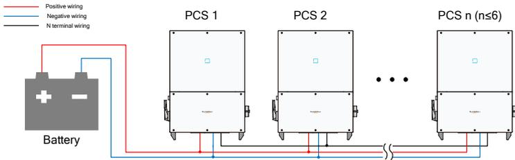
The wiring between the two DC parallel machines is shown in the figure below, and the wiring is the same as the DC wiring:
