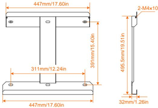
**Fig. 5-1** Dimensions of the bracket (figures in inch)
