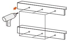
**Step 5** Secure the bracket to the metal frame firmly with the supplied fastener. The torque of the fastener nut is 35 N·m.
