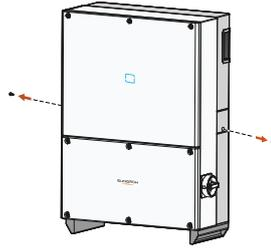
**Step 8** Clasp the groove (near the cover plate of the fan) on the back of the PCS by your fingers and pull out the slot of the fan.
