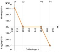
Fig. 12-2 Reactive Power Regulation Curve in Q(u) Curve ("AU" for example)
