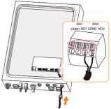
5. Fasten the swivel nut and connect the other end of the cable to the original edge of the AC contactor.
