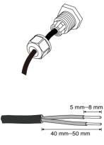
4. Plug the wires into **DO** terminals without tool tightening.
