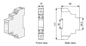
Fig. 2-4 single-phase Meter Dimensions (unit: mm)
