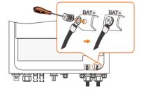
5. Loosen and remove the screw sets on the **BAT+** and **BAT-** terminal blocks.
