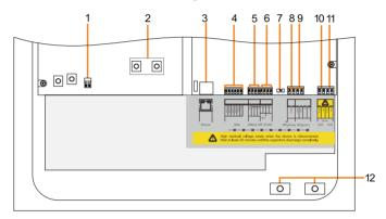
Fig. 6-2 Configuration Circuit Board Inside the Inverter
