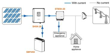
Fig. 2-7 Inverter Application in an Off-grid System
