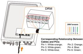
5. Fasten the swivel nut and connect the other end to the DRED.
