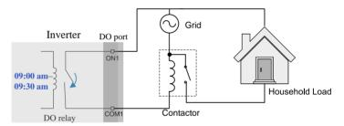
Fig. 10-2 DO Operation in Timer Control
