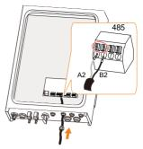
When the length of RS485 cable is longer than 100 m, push the 120 Ohm (2) switch to "ON" to ensure stable communication, as shown below.
