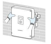
Secure the inverter with two M5 screws and washers. (3.0 N·m)
