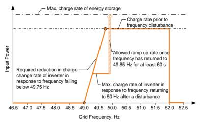
Fig. 12-6 Frq-Watt Mode for Under-frequency Conditions
