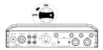
Check the cable connection of the PV strings for the correct polarity and that the open circuit voltage does not exceed the inverter input limit of 600 V, even under the lowest operating temperature. Refer to the module specification supplied by the module manufacturer for detailed information.
