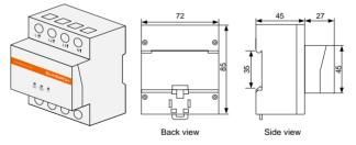
Fig. 2-5 Three-phase Meter Dimensions (unit: mm)
