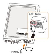
5. Fasten the swivel nut and place the temperature sensor next to the lead-acid battery.
