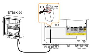
4. Plug the wires of the DI cable into terminals **DI1**, **DI2**, **DI3** and **VDD** according to the marks without tool tightening, as shown below.
