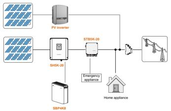
Fig. 2-8 Retrofitting the Existing PV System
