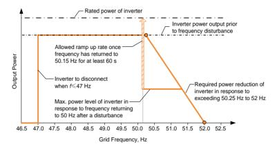
Fig. 12-5 Frq-Watt Mode for Over-frequency Conditions
