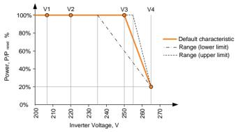
Fig. 12-3 Volt-Watt Response Curve ("AU" for example)
