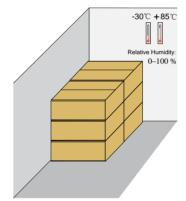
Fig. 4-3 Example of Inverter Storage
