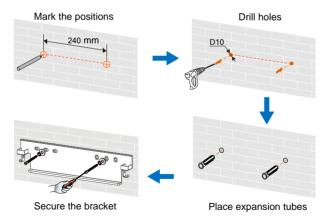
Note that the depth of the holes should be about 70 mm. Be sure to adhere to the screw assembly sequence: self-tapping screw, spring washer, fender washer and bracket.
