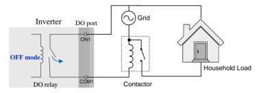
Fig. 10-3 DO Operation in ON/OFF Control
