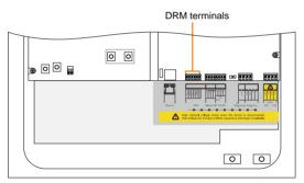
The modes from DRM0 to DRM8 are supported by the inverter and the information is marked on the label located near the DRM terminals.
