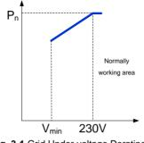
Fig. 3-1 Grid Under-voltage Derating
