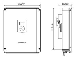
Fig. 2-2 Dimensions (unit: mm)
