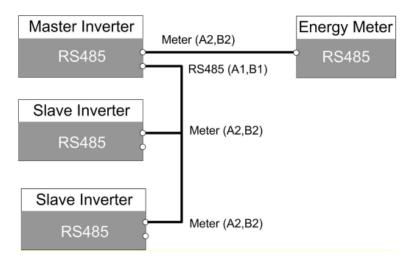
The location of RS485 (A1, B1) and Meter (A2, B2) is shown in the following figure.
