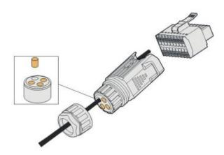
**Step 4** Remove the cable jacket and strip the wire insulation.
