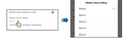
**Step 5** Switch on the "Master-slave operation mode", change the master slave setting to "Master" or "Slave#" correspondingly, and input the total number of master and slaves in the chain.
