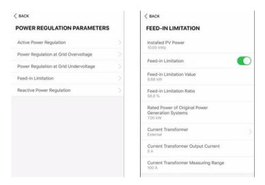
In the Installed PV Power, put 20kW if there are 2 SH10RT inverters.
