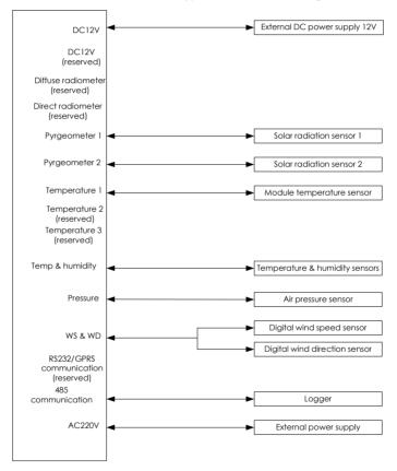
Note: Two types of power supply ports are reserved on the main control box, that is, the DC power supply port and the AC power supply port. On site, the user can select either one to supply power.
