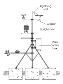
Proceed as follows to install the environment monitoring device:
