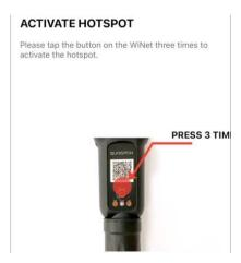
Once complete, the SG-xxxx Wi-Fi will be available in the Wi-Fi list and local access feature can then be utilised.
