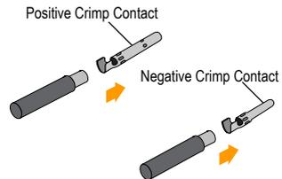
**Step 3** Lead the cable through cable gland, and insert into the insulator until it snaps into place. Gently pull the cable backward to ensure firm connection. Tighten the cable gland and the insulator (torque 2.5 N·m to 3 N·m).
