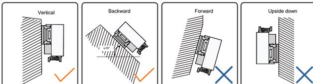
In case the installation site is a level surface, mount the inverter to the horizontal-mounting bracket to meet the mounting angle requirements, as shown in the figure below.
