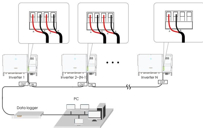
**Fig. 5-4** Multi-inverter inverter communication system
