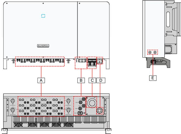
**Fig. 5-1** Wiring terminals
