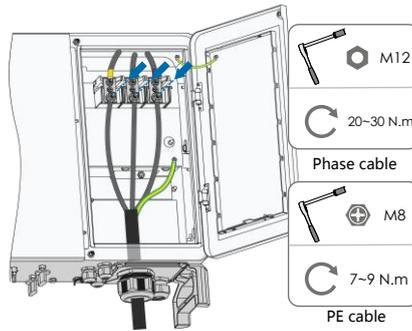
**Step 8** Gently pull the cable backwards to ensure firm connection, and fasten the swivel nut clockwise.
