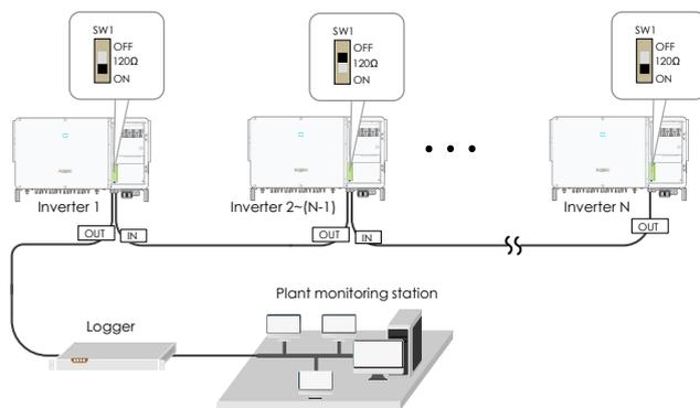
**Fig. 5-5** Configuration of dip switch ( $N \geq 15$ )
