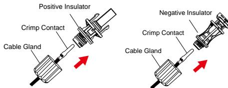
**Step 4** Check for polarity correctness.
