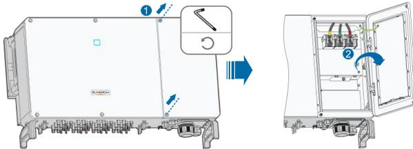
**Step 3** Keep the wiring compartment opened during wiring through the limit lever attached to the cover.
