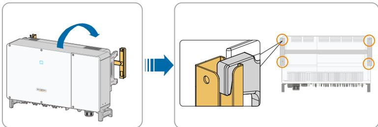
**Step 7** Fix the inverter with two M6×65 screws.
