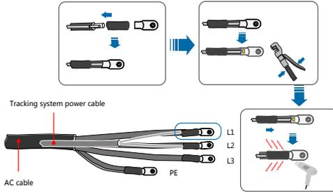
**Step 5** Secure the wires to corresponding terminals.
