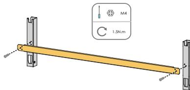
**Step 2** Level the assembled mounting-bracket by using the level, and mark the positions for drilling holes on the PV bracket. Drill the holes by using a hammer drill.
