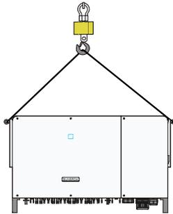
**Step 5** Remove the lifting rings and reassemble the sealing screws released in Step 1.
