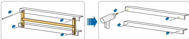
**Step 3** Secure the mounting-bracket with bolts.
