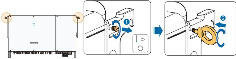
**Step 3** Lead the sling through the two lifting rings and fasten the tie-down strap.
