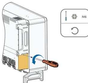
**Step 3** Press the hump of the latch hook, unplug the cable connection joint outwards, and loosen the screw on the fan holder.
