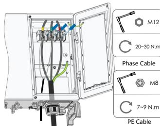
**Step 6** Gently pull the cable backwards to ensure firm connection, and fasten the swivel nut clockwise.
