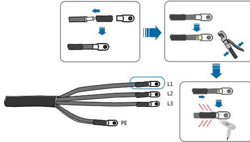
**Step 7** Secure the wires to corresponding terminals.
