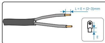
**Step 4** Crimp tracking system power wires together with two phase wires in the AC cable. Other AC wires are crimped independently.
