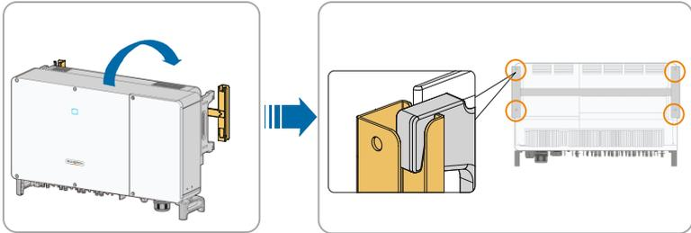
**Step 8** Fix the inverter with two M6×65 screws.
