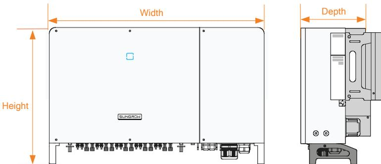
**Fig. 2-3** Dimensions of the Inverter (in mm)
