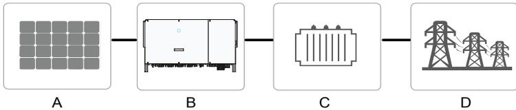
Fig. 2-1 Inverter application in PV power system
