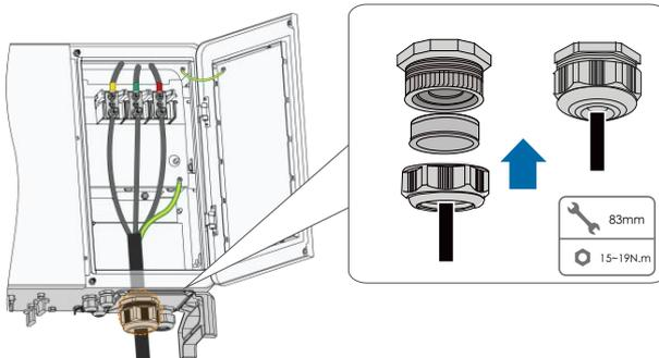
If the PE cable is an independent single-core cable, it is inserted into the cabinet through the standby grounding terminal.
