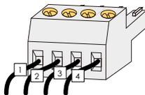
**Step 4** Insert the terminal base into the corresponding terminal block.
