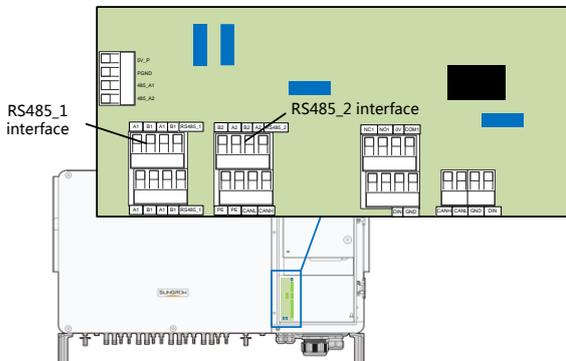
The inverter is equipped with two groups of RS485 communication interfaces for external communication connection. Both the two groups of interfaces can be connected to the data collector (Logger), to achieve data exchange with PC or other monitoring devices.
