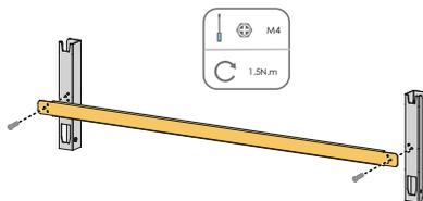
**Step 2** Level the assembled mounting-bracket by using the level, and mark the positions for drilling holes on the installation site
