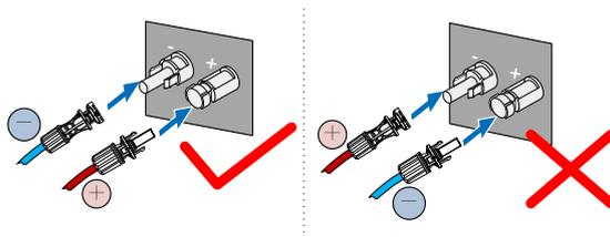
**Arc or contactor over-temperature may occur if the PV connectors are not firmly in place, and damage caused shall not be covered by the warranty.**
