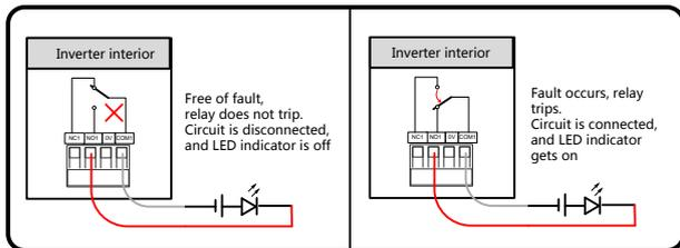
Fig. 5-6 Normal open contact
